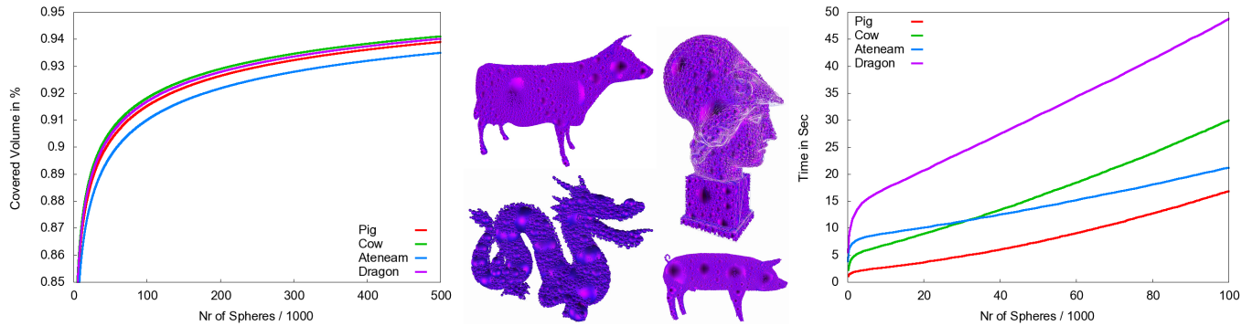
Figure 2: The space filling rate of our sphere packing algorithm (left). The models used for the timings: A cow, a pig, a bust and a dragon (middle). Timings for different objects on a Geforce GTX480 (right; please note that the code is not optimized yet).
